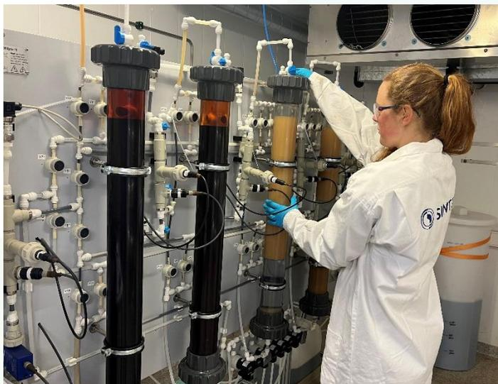
The vanillin-phenolic process is semi-continuous in design. Peroxidarbonate (PODIC<sup>®</sup>) is used as the oxidizing agent and generated from sodium carbonate in an electrochemical cell with boron-doped diamond electrodes, which was developed by our project partner CONDIAS GmbH. A variety of feed modes offers the possibility to analyse different ratios and distributions of lignin feed and PODIC<sup>®</sup> stream.
